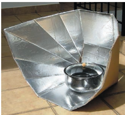
Figure 8.22: Improvised solar cooker A. Made of folded sleeping pad and box cooker. (Source: http://solarcooking.org/plans/ )
